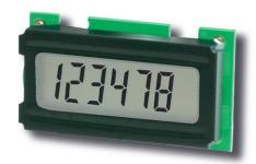
Type 192 is a single channel counter module for PCB mounting, with a large voltage range of 8 up to 28 V DC and a 6-digit LCD
